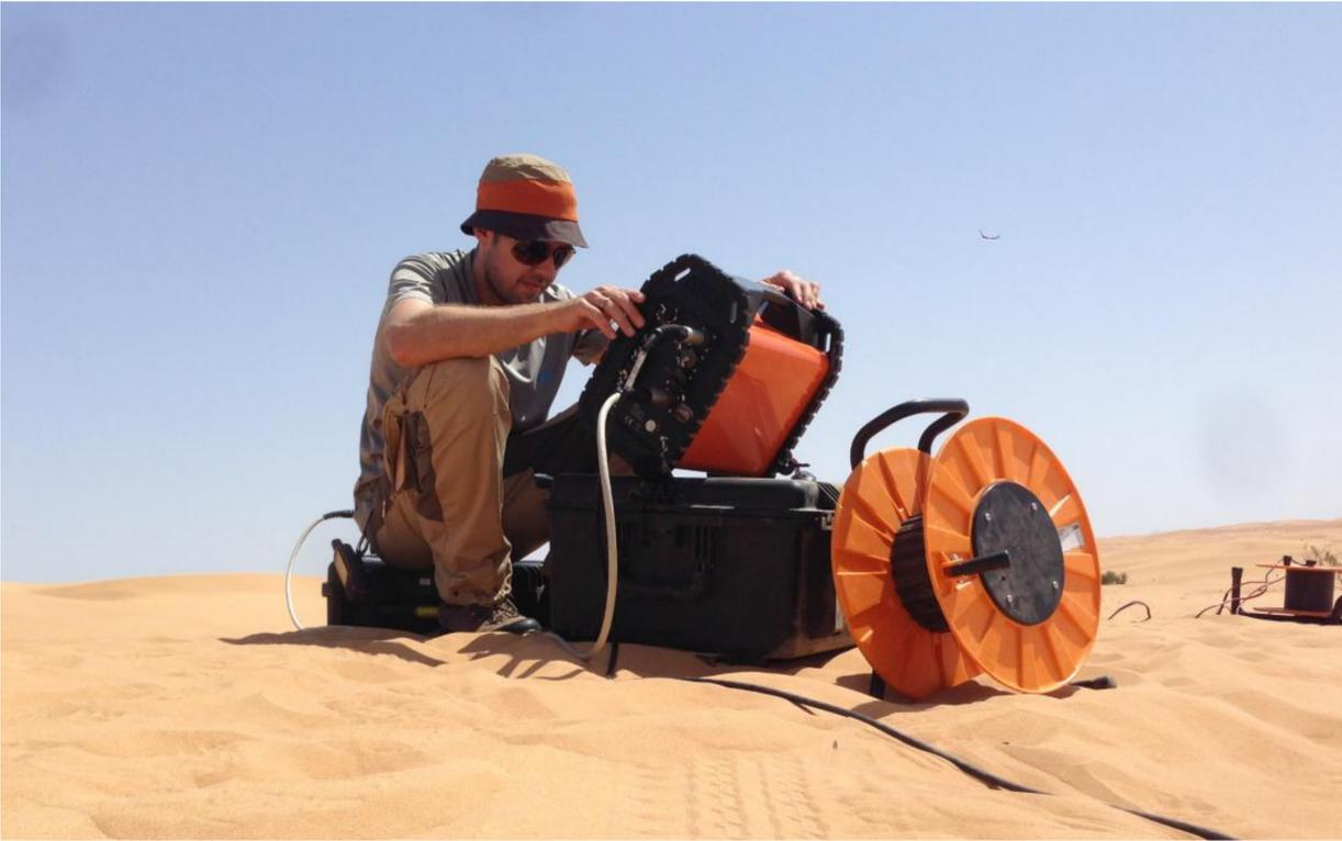
Figure 3 WalkTEM system for single site TDEM measurements
